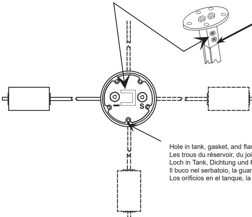
Self tapping screws penetrate directly into and through channel to secure the channel to the flange.
