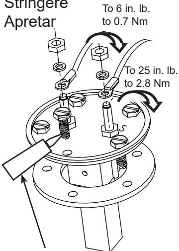
Apply thread sealer to screw threads before installing in tank.
